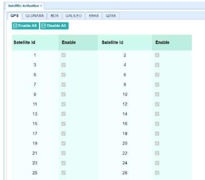
The screenshot shows the 'Satellite Activation' window with tabs for GPS, GLONASS, BDS, GALILEO, SBAS, and QZSS. Below the tabs are 'Enable All' and 'Disable All' buttons. A table lists satellite IDs from 1 to 26, with each ID having an 'Enable' checkbox that is checked.
